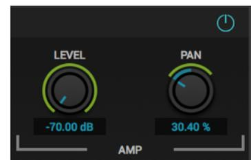
The little blue icon in the top right corner of the chain (above the Pan knob) lets you activate/deactivate the whole chain. When this button is off, the chain will be bypassed : its controls will be disabled and the chain will not be processed at all, saving some precious CPU cycles. It is recommended to fully deactivate a chain this way when not in use instead of lowering its output level to reduce the processing power needed by the plugin.
