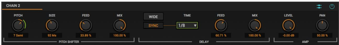
The three effect chains are at the heart of Incipit. They act as three layers that operate on the input signal. Each chain is made of three modules : a Pitch Shifter, a Delay and an Amplifier section. The signal flows through them in the same order as they appear on the panel.
